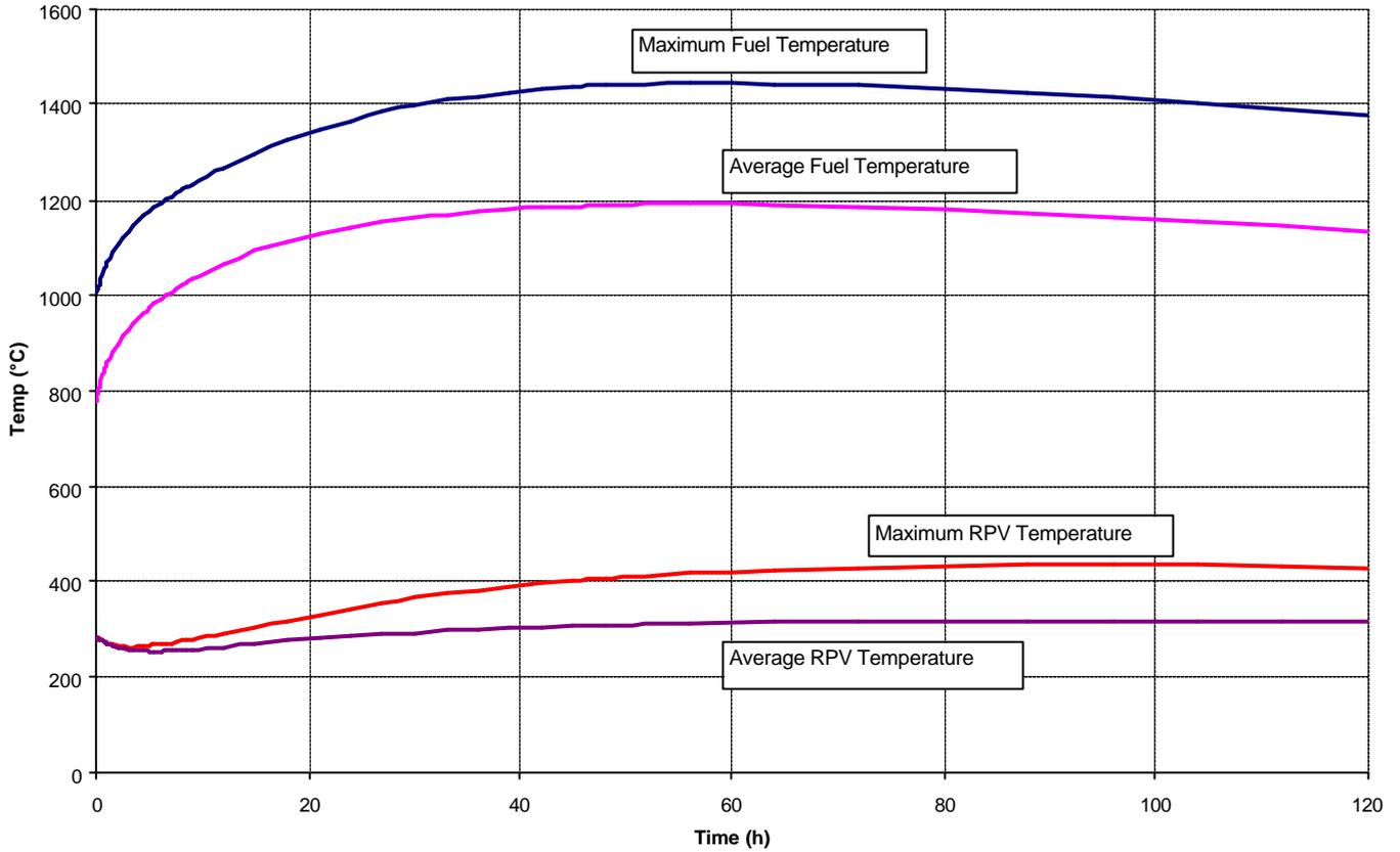
The figure shows the temperature of the hottest part of the fuel and overall average after a total loss of coolant
