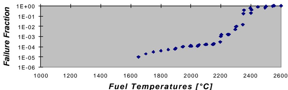
**The figure shows the performance of the fuel under extended periods at high temperatures**
